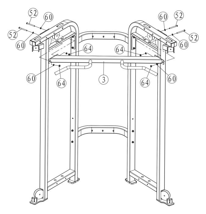
STEP 2 Attach Main Beam (3) to Left and Right Frames (1 & 2) using Bolts M10X105 (52), Washers M10 (60), and Nylon Nuts M10 (64).
